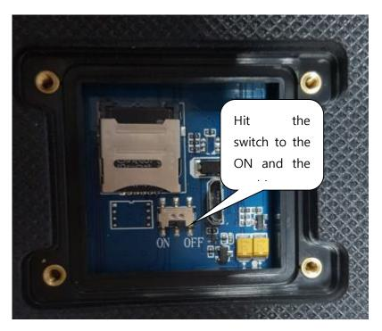
2. Install the SIM and turn on the battery switch, cover the bottom cover, on the good screw
